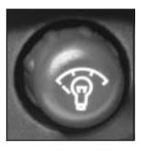
Press the knob located next to the exterior lamps knob to extend it.
